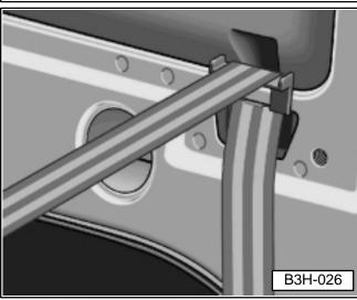
Guide tether strap under rear seat head restraints through guide as shown, and route to tether anchors in luggage compartment.
