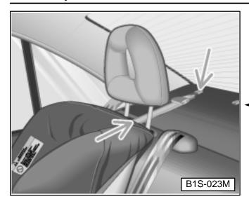
A tether anchor is used to connect the child restraint (CR) tether strap to the vehicle. A tether is a straight or V–shaped strap that attaches the top part of a CR to special anchorage points in the vehicle.
