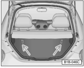
Illustration shows seat back with tether anchors for New Beetle.
